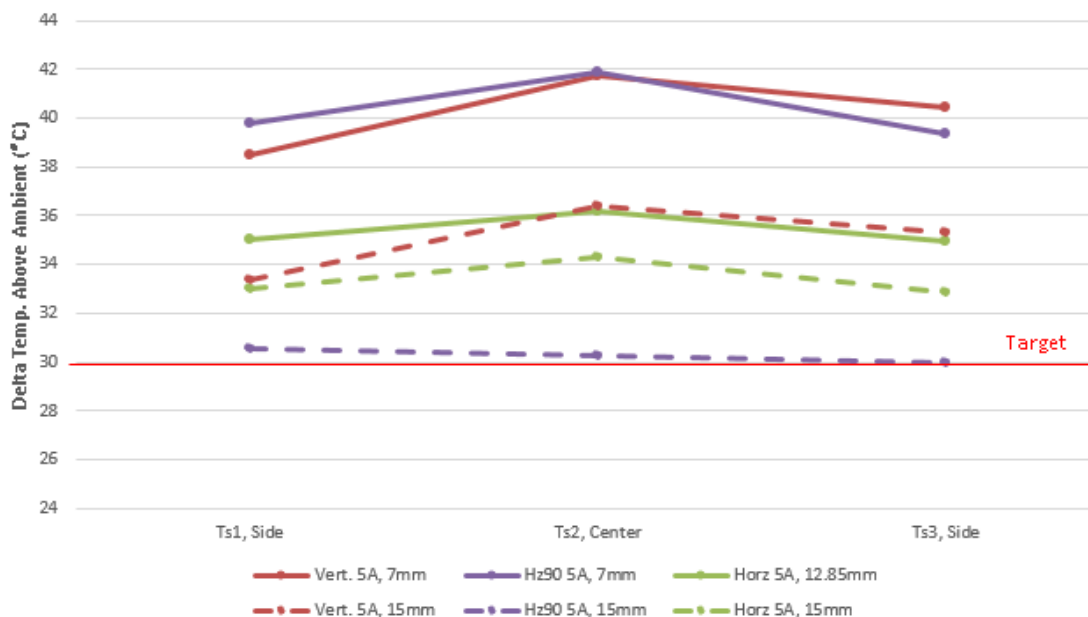
Figure D-13 USB 3.2 Dual-Lane 5A Active Cable in a 3-Port Configuration
